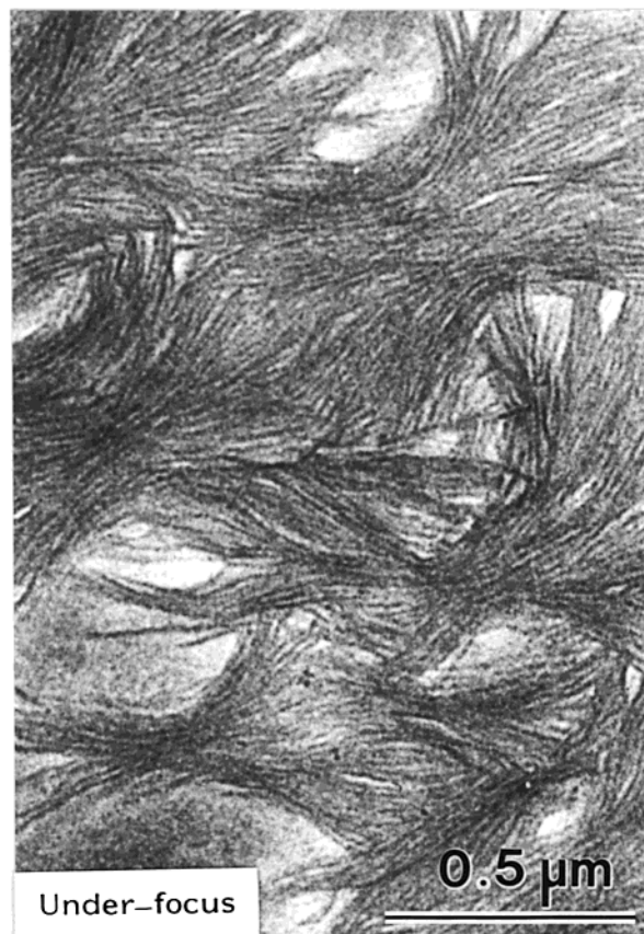
Figure 2. Bright-field image of an i-PS thin film which was crystallized at 170 °C for about 60 min. This image was obtained by the defocus contrast method, 28 namely, taken at a fairly large amount of objective-lens defocus (at an under-focus of about 40 μm at 200 kV).
